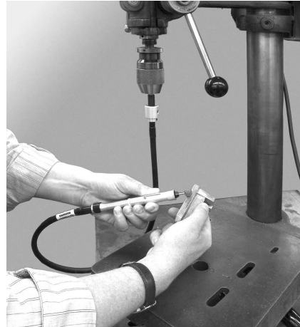
The Flexade converts a Drill Press into a flexible shaft machine. It is shown here with an H.8 handpiece that is available separately.
